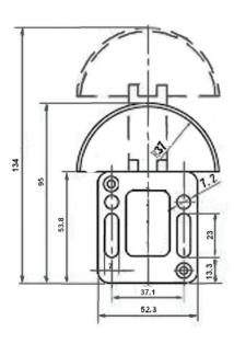
Arch profiles made of UHMW, PE Max load (25C) 130N
